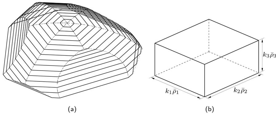
**Fig. 3:** Examples of the workspace of the Tripteron for (a) relatively short legs (only the upper part is shown) and (b) relatively long legs.
