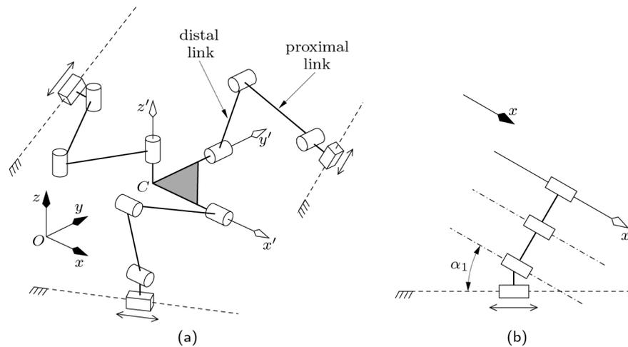
**Fig. 1:** Schematics of (a) the Tripteron and (b) the projection of one of its legs onto a plane parallel to the axes of the leg's revolute joints and the direction of the leg's prismatic joint.
