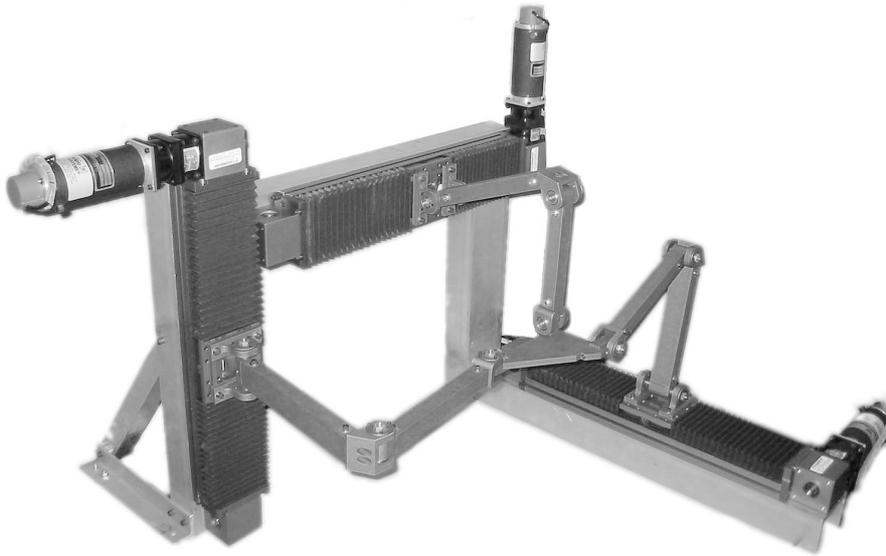
**Fig. 6:** The prototype of the Orthogonal Tripteron.
