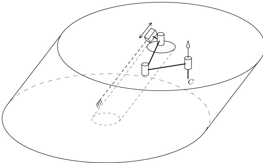
**Fig. 2:** Schematic of the vertex space for one of the Tripteron's legs.
