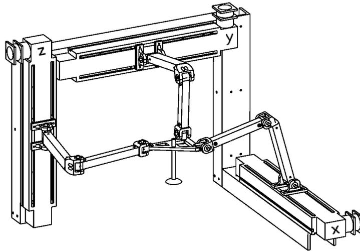
**Fig. 5:** A CAD model of the Orthogonal Tripteron.
